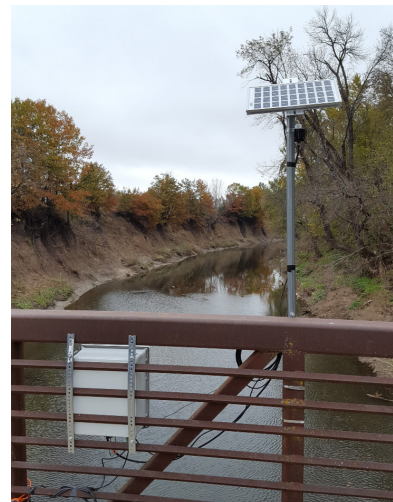
Solar power surface water monitoring station
